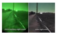
Built with 4 color night vision camera, it can output HD color video at total darkness environment. Real-time images can be displayed in single view or two, even 4, etc. It can be powered by the vehicle or its built-in battery. APP in the phones or pads can connect it with WIFI for remote checking.
